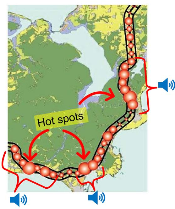
The deterrent sound was designed to be played back from a train. A 55-km-long section was chosen for the test out of the 135-km-long line. For the playback, an audio system was installed in a train and a speaker was settled at both ends of the train.
