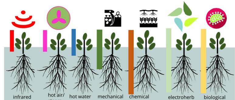
Most of the alternative methods target only the upper part of the plants. Perennial plants with deep root system and rhizomes will regrow. Chemicals are able to penetrate the plant and damage also roots and root systems. Electric high voltage reaches the root systems when applied on the upper plant part. The method is still under development. Biological control with microorganism can reach the roots system and is the only method, beside some herbicides, which can also effect seed germination.
